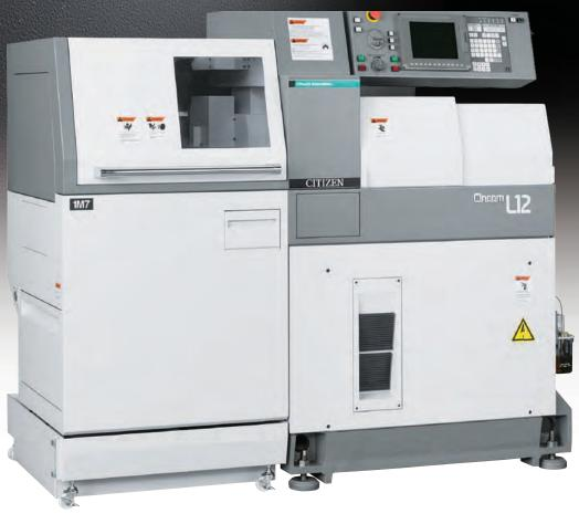
Machining using a guide bushing is a useful method for small diameter workpieces. However, using a guide bushing with short workpieces produces more material waste which increases material costs. The optimum machine configuration differs depending on the workpiece to be machined, and up until now a variety of different machines
