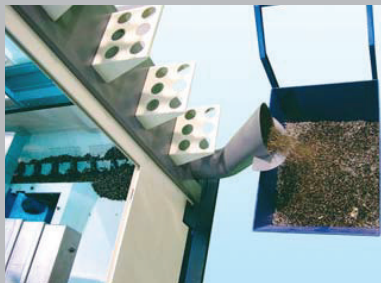
A simple but efficient removal mechanism can easily convey the chips outside of the machine.
