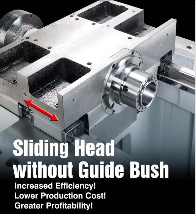
Spindle head moves on two precision linear ways combined with extra large span between ways, exhibiting outstanding stability and high positioning accuracy.
